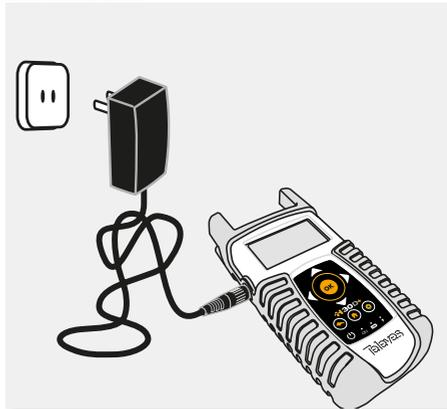
When external power is supplied, the battery management system automatically controls the charging process.
